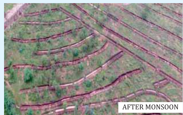
Continuous Contour Trench (CCT) and Deep CCT [IWMP-3 (2010-11), Latitude and longitude - 25.114869 & 74.06376, Gram panchayat - Akhodiya khed Block - Rajsamand, District : Rajsamand, Rajasthan]
